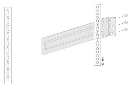
c) Repeat Step 3 to attach the other slider rail to the other side of the rack.
