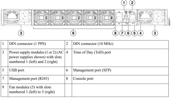
The following figure shows the switch features on the side of the chassis.
