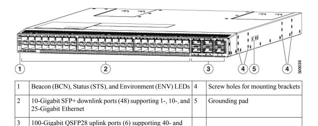
To determine which transceivers, adapters, and cables are supported by this switch, see the Cisco Transceiver Modules Compatibility Information document.
