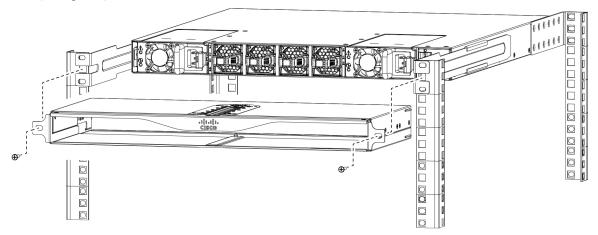
c) Tighten the 10-32 screws to 20 in-lb (2.26 N·m) or tighten the 12-24 screws to 30 in-lb (3.39 N·m) of torque.
