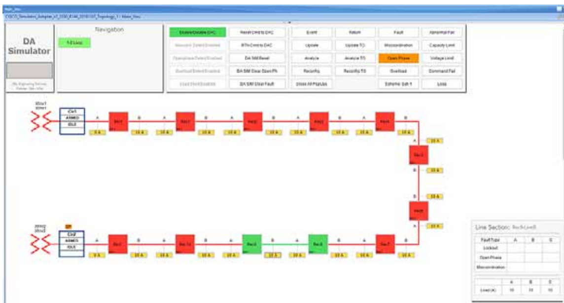
Figure 190 Open Phase clear fault
