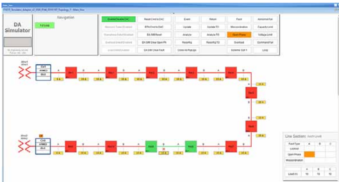
Figure 189 Open Phase FLISR state
