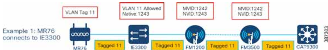
Figure 30 VLAN configuration for MR connects to IE3300
