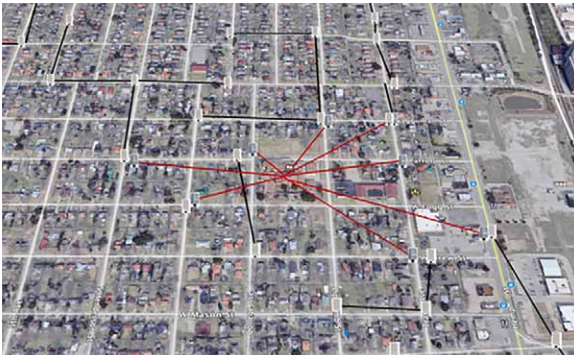
Figure 6 Final mesh radio network path
