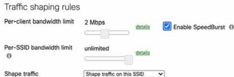
Figure 25 Traffic shaping rules configuration for general public free Wi-Fi SSID
