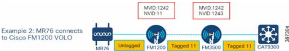
Figure 31 VLAN configuration for MR connects to Cisco FM 1200 Volo
