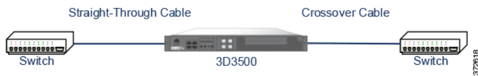
Figure 3-1 Straight-Through Bypass Connection Cabling
