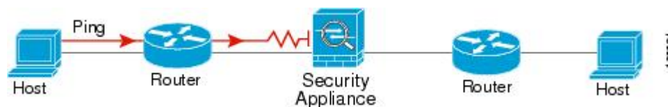
Figure 63: Ping Failure Because the ASA is Not Translating Addresses
