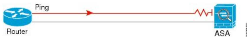
Figure 62: Ping Failure Because the ASA Has No Return Route
