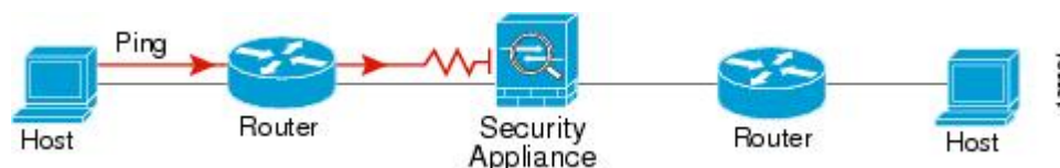
Figure 93: Ping Failure Because the ASA is Not Translating Addresses
