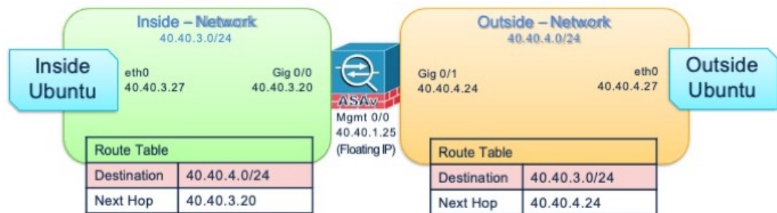
Figure 65: Sample ASAv on OpenStack Deployment
