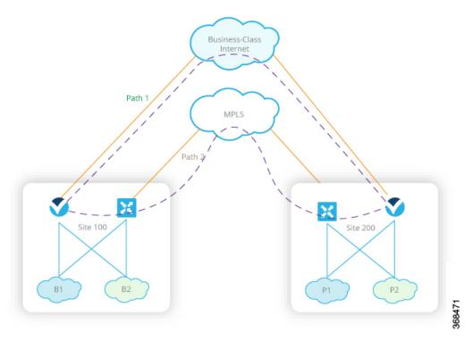
Each Cisco IOS XE SD-WAN device supports up to eight TLOCs, allowing a single Cisco IOS XE SD-WAN device to connect to up to eight different WAN networks. This capability allows path customization for application traffic that has different needs in terms of packet loss and latency.
