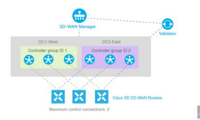
You configure the three Cisco SD-WAN Controllers in DC1-West with controller group identifier 1:
