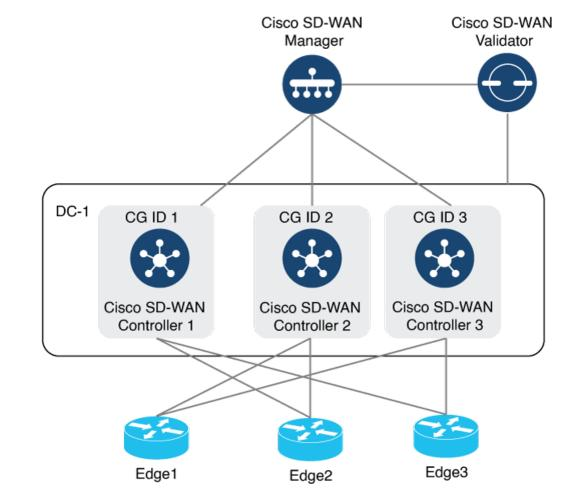
To display the control connections with the Cisco SD-WAN Controllers, use the **show sdwan control connections** command. The last column on the output, **Controller Group ID**, lists the Cisco SD-WAN Controller group that a router is in.
