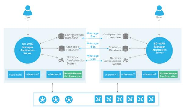
with a Cisco Catalyst SD-WAN software process (vdaemon) running on each core. In addition, the VM stores the actual configuration for the Cisco SD-WAN Manager server itself.
