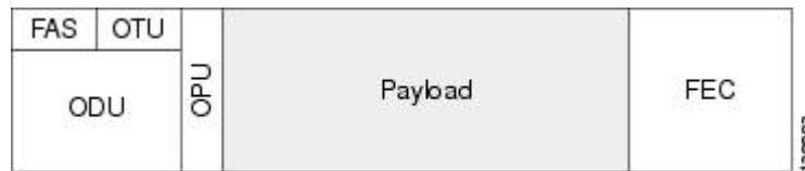
Figure 5: OTN Optical Channel Structure
