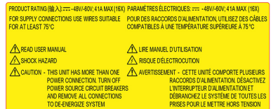
Figure 1: Rating Label for NCS 4000 FCC DC Chassis
