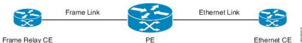
Figure 1: Frame Relay-Ethernet Local Switching Topology
