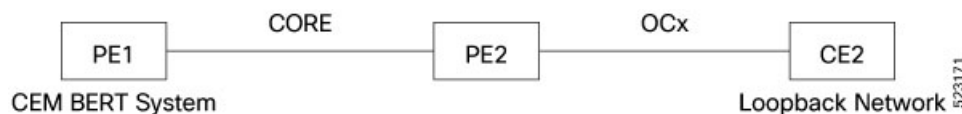
Figure 8: Configuring System CESoP NxDS0 BERT with System Direction and Speed on PE1 and Loopback as Network on CE2
