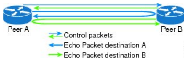
Figure 19: BFD Asynchronous Mode With Echo Packets
