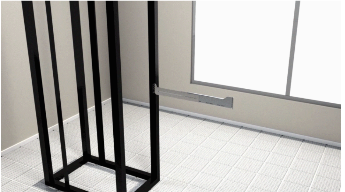
Figure 11: Four Post Slider Integration in the 19" Rack
