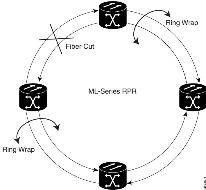
In case of a ring failure, the ML-Series cards connected to the failed section of the Cisco proprietary RPR detect the failure through the SONET/SDH path alarms. When any ML-Series card receives this path-AIS signal, it wraps the POS interface that received the signal.
