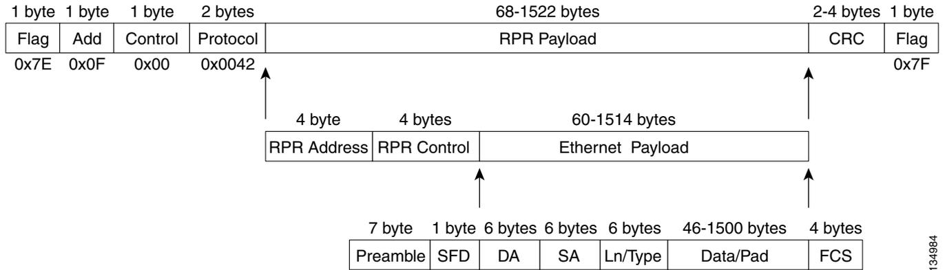
The Cisco proprietary RPR framing and header includes a number of fields, including four bytes for source and destination station information and another four bytes for control and quality of service (QoS). [Figure 17-4](#) illustrates the Cisco proprietary RPR frame format. [Table 17-1](#) defines the most important fields.
