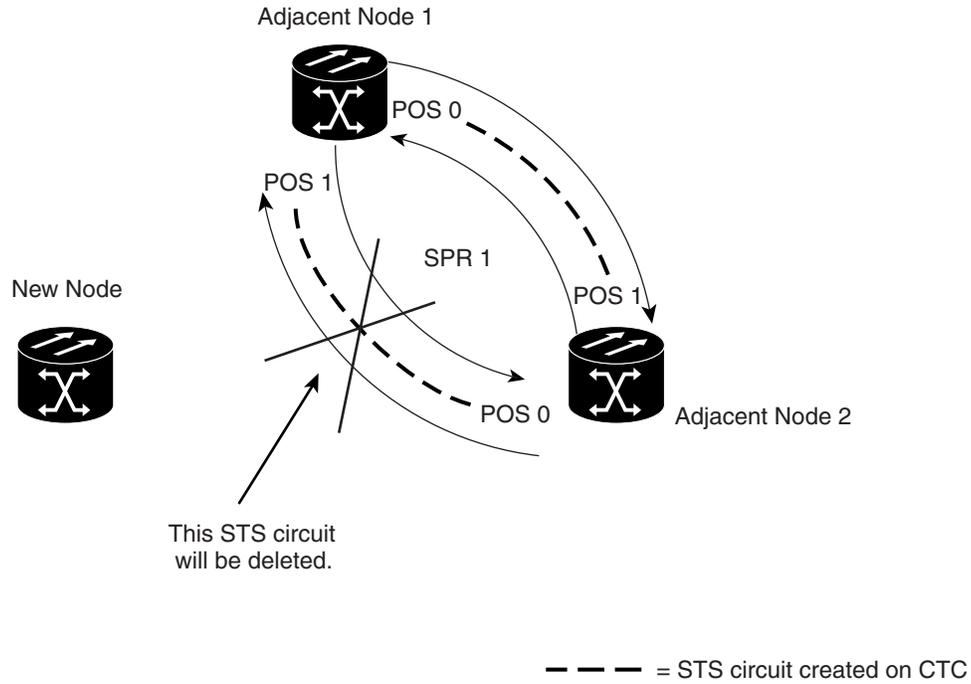
**Figure 17-10 Three Node Cisco Proprietary RPR After the Addition**
