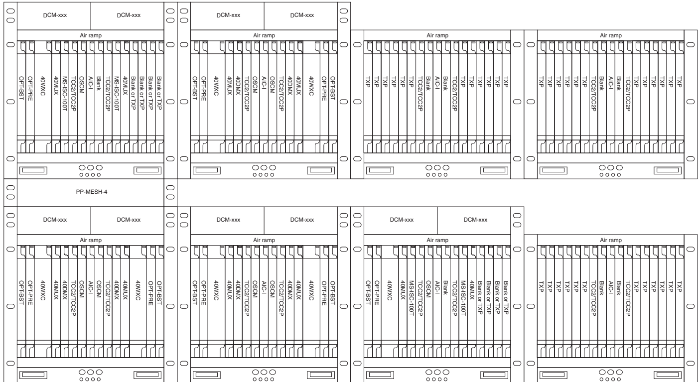
Figure 9-31 Four-Degree Protected Line Termination Mesh Node Layout
