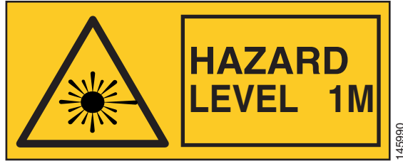
Figure 4-2 Hazard Level Label
