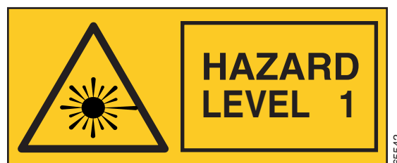
Figure 8-2 Hazard Level Label
