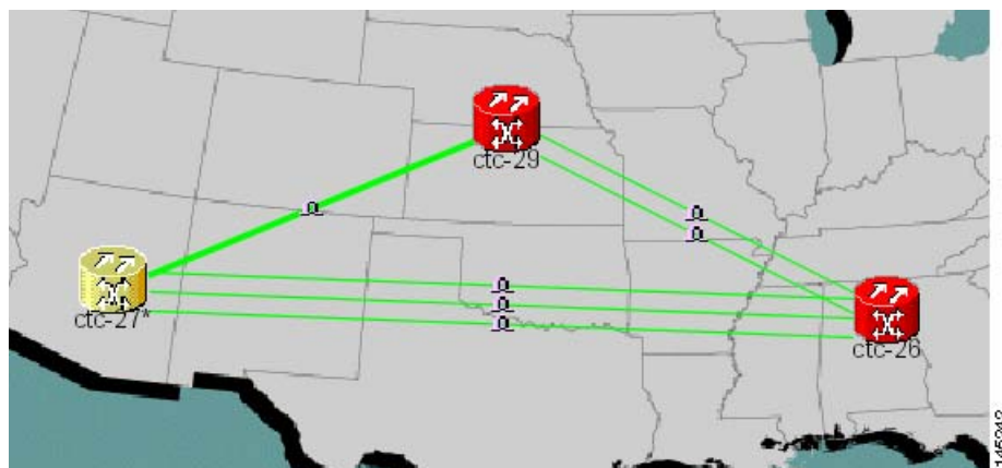
Figure 21-15 Network View with Local Link Consolidation
