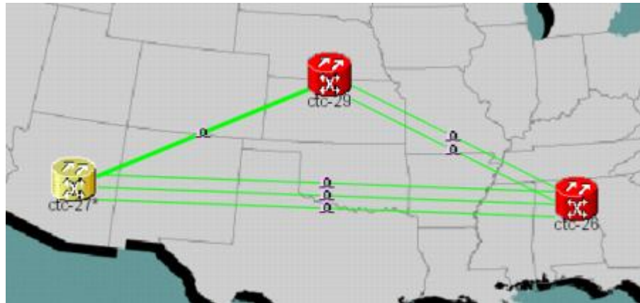
Figure 3: Network View with Local Link Consolidation
