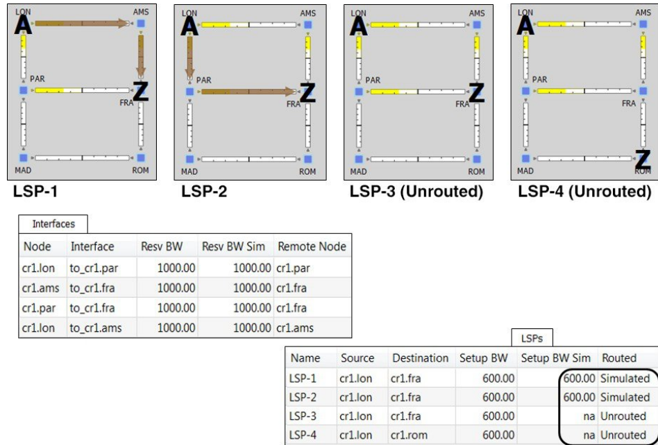
Figure 57: Simulated Routing Using Reservable Bandwidth Constraints
