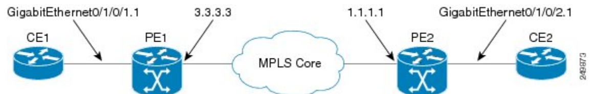
Figure 1: VPLS with BGP autodiscovery and BGP signaling
