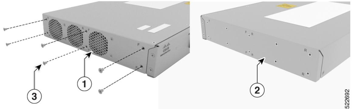
Figure 31: Remove Screws from the Sides of the Chassis
