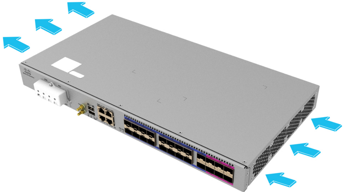
Figure 16: Airflow Side View of Cisco N540-6Z18G-SYS-A/D Router from Front to Left
