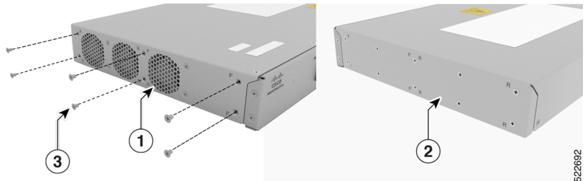
Figure 38: Remove Screws from the Sides of the Chassis
