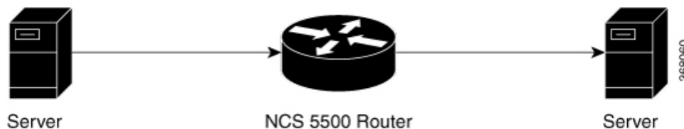
Figure 12: Topology for ERSPAN Egress Rate Limit
