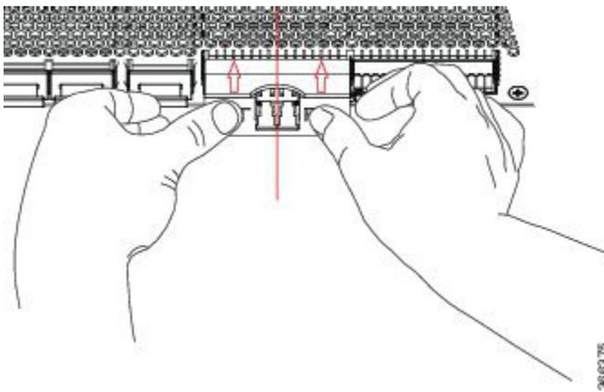
**Step 5** When you are ready to attach the network cable interface, remove the dust plugs and inspect and clean fiber connector end faces, and then immediately attach the network interface cable connectors into the CFP2 module optical bores.
