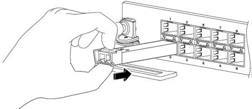
**Note** When installing an SFP or SFP+ module, you should hear a click as the triangular pin on the bottom of the SFP module snaps into the hole in the receptacle. This click indicates that the module is correctly seated and secured in the receptacle. Verify that the SFP modules are completely seated and secured in their assigned receptacles on the line card by firmly pushing on each SFP module.
