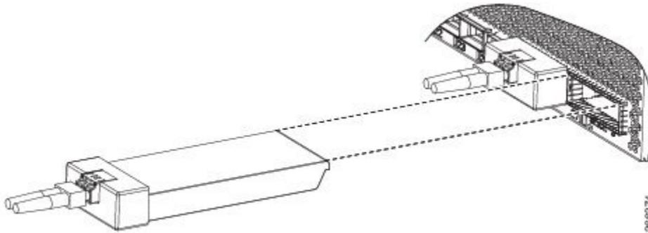
**Step 3** Slide the CFP2 module in until the EMI gasket flange makes contact with the line card faceplate.
