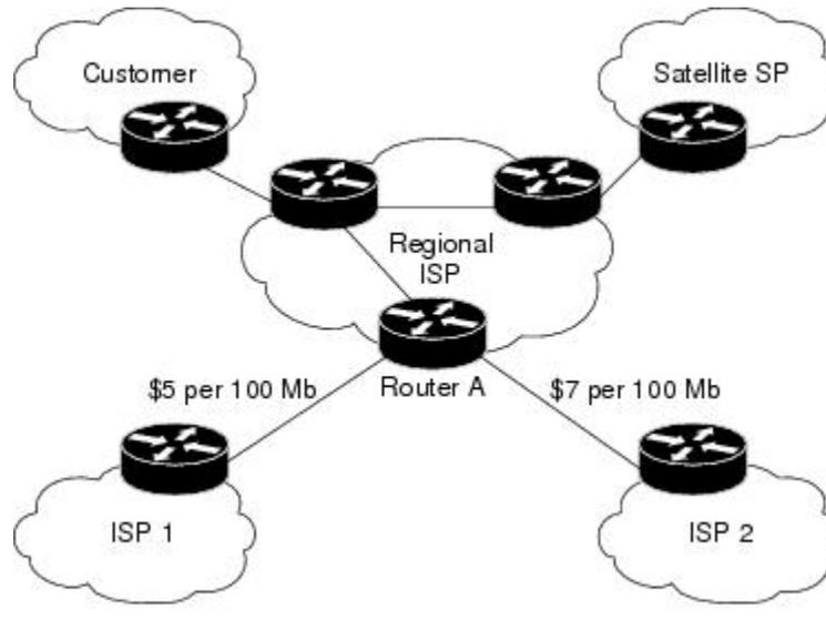
Based on the specified routing policy, BGP policy accounting assigns each prefix a traffic index (bucket) associated with an interface. BGP prefixes are downloaded from the RIB to the FIB along with the traffic index.
