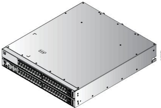
Figure 4: Cisco NCS 5002 - Front (Port Side) View
