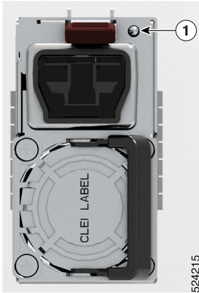
Figure 15: Power Supply LED - 8212-48FH-M Chassis
