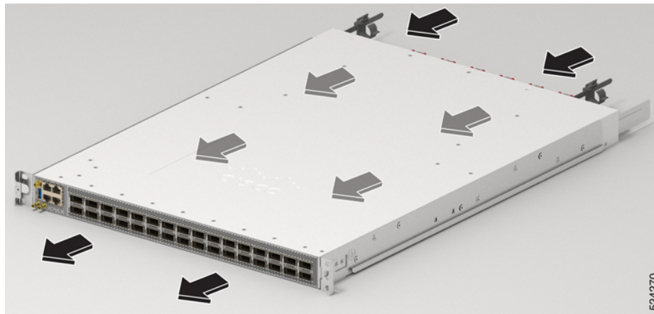
Figure 13: Airflow Direction for Cisco 8712-MOD-M Router in PSI Configuration
