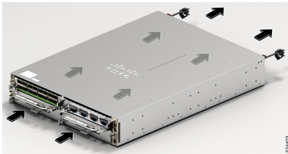
Figure 13: Airflow Direction for Cisco 8712-MOD-M Router in PSI Configuration
