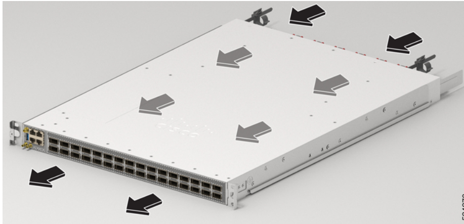
Figure 5: Airflow Direction for Cisco 8712-MOD-M Router in PSI Configuration
