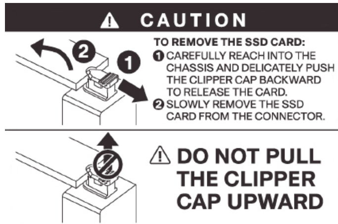
Figure 12: SSD Card Removal Instructions
