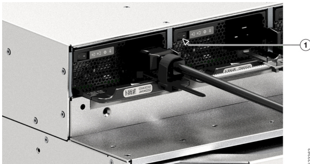
Figure 30: Power Switch in Off Position - PSU3.2KW-ACPI
