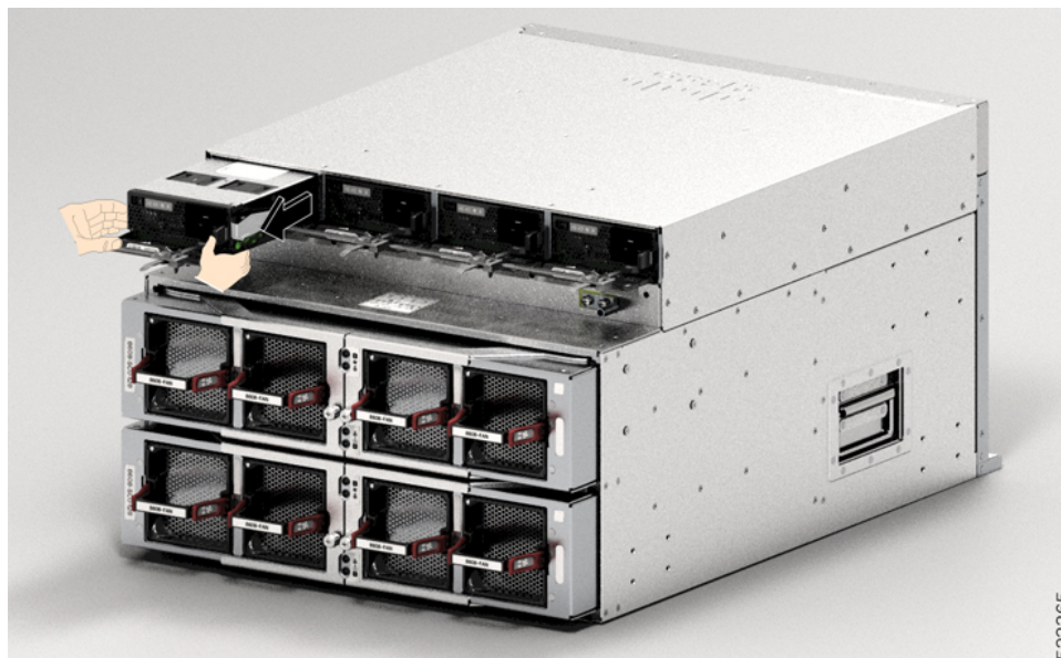
Figure 121: Slide the PSU Out - PSU3.2KW-ACPI
