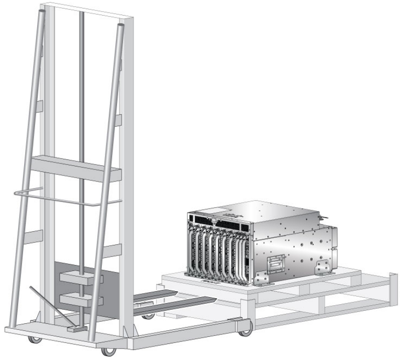
Figure 18: Align the Lifting Device in Front of the Chassis on the Pallet
