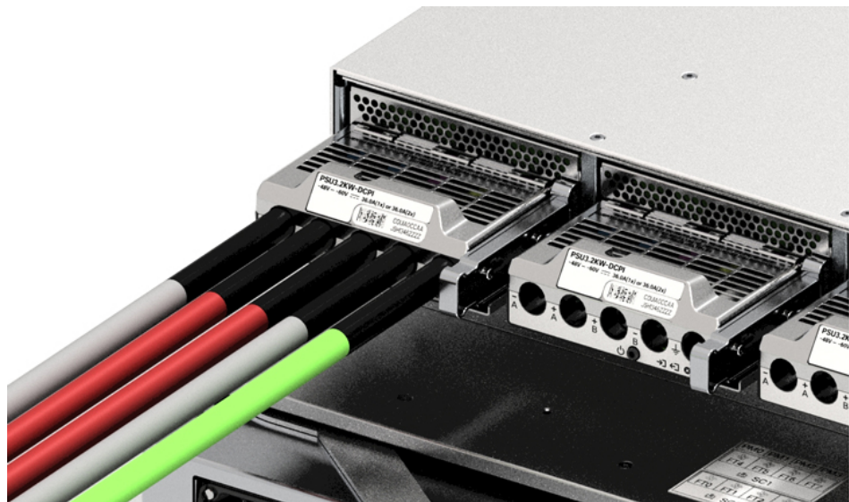
Figure 124: Open Terminal Block Cover
