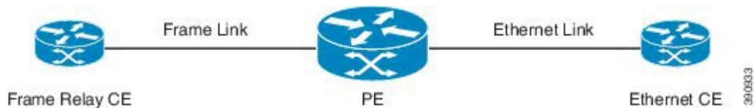
Figure 3: Frame Relay-Ethernet Local Switching Topology
