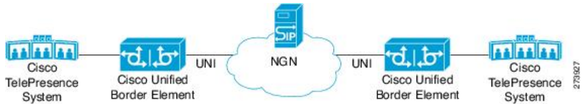
Figure 1: Cisco NGN with CCUBE providing UNI interface
