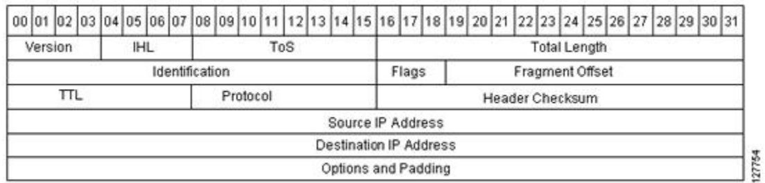
Figure 34: IP Packet Header Fields
