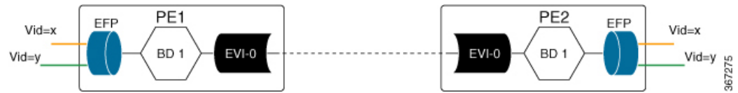
Figure 48: VLAN Bundle Service Interface
