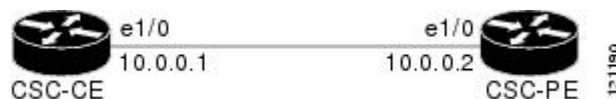
Figure 22: Configuration for Peering with Directly Connected Interfaces Between CSC-PE and CSC-CE Routers
