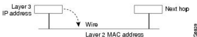
Figure 4 Layer 3-to-Layer 2 Mapping
