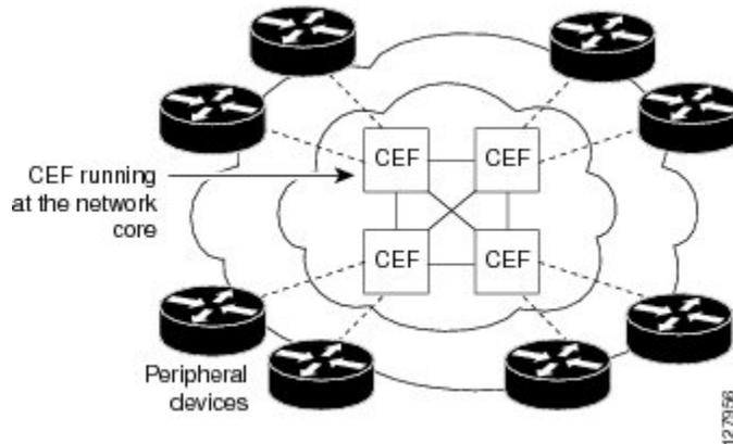
Cisco Express Forwarding in platforms at the network core provides the performance and scalability that networks need to respond to continued growth and steadily increasing network traffic. Cisco Express Forwarding is a distributed switching mechanism that scales linearly with the number of interface cards and the bandwidth installed in the router.
