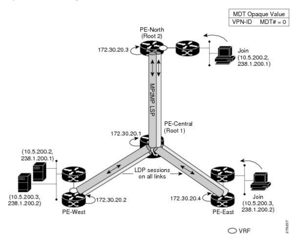
This configuration is consistent for every PE device participating in the same VPN ID. The **vpn id 100:2** command replaces the MDT group address used with the mGRE transport method. To provide redundancy, two default MDT trees are statically configured, rooted at P-Central and PE-North. The selection as to which MP2MP tree the default MDT will use at a particular PE device is determined by Interior Gateway Protocol (IGP) metrics. An MP2MP LSP is implicit for the default MDT.
