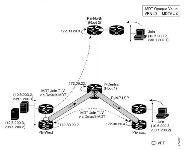
The sample output in this section displays the data MDT configuration for all the PE devices. The **mdt data** commands are the only additional commands necessary. The first **mdt data**command allows a maximum of 60 data MDTs to be created, and the second **mdt data**command sets the threshold. If the number of data MDTs exceeds 60, then the data MDTs will be reused in the same way as they are for the mGRE tunnel method (the one with the lowest reference count).
