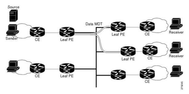
Data MDTs are created only for (S, G) multicast route entries within the VRF multicast routing table. They are not created for (\*, G) entries regardless of the value of the individual source data rate.
