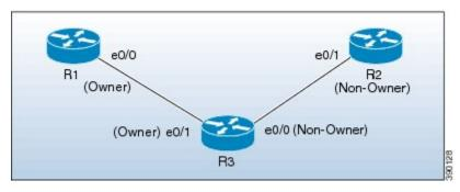
In this topology, device R3 is incorrectly inserted between the devices R1 and R2, with its interfaces swapped. The conflict arises due to incorrect insertion, as given below:
