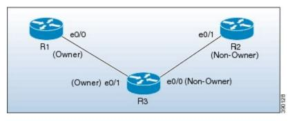
In this topology, device R3 is incorrectly inserted between the devices R1 and R2, with its interfaces swapped. The conflict arises due to incorrect insertion, as given below:
