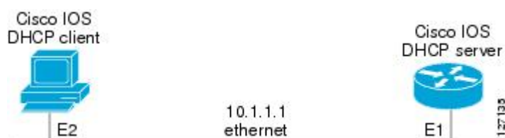
Figure 2: Topology Showing DHCP Client with GigabitEthernet Interface
