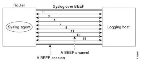
Channels are identified as 1, 3, 5, 7, 9, 11, 13, and 15. The number of available channels (eight) was designed to correspond to the number of severity levels of classic RFC-3164 syslog messages (0 to 7). Message
