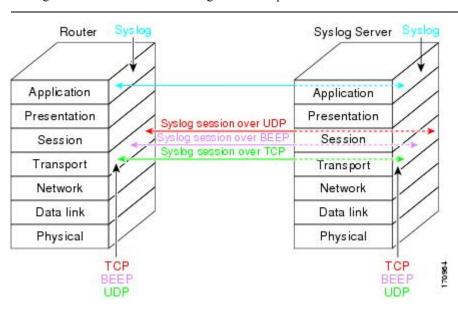
The figure below shows multiple syslog sessions from a single syslog agent to different hosts using UDP, TCP and BEEP.
