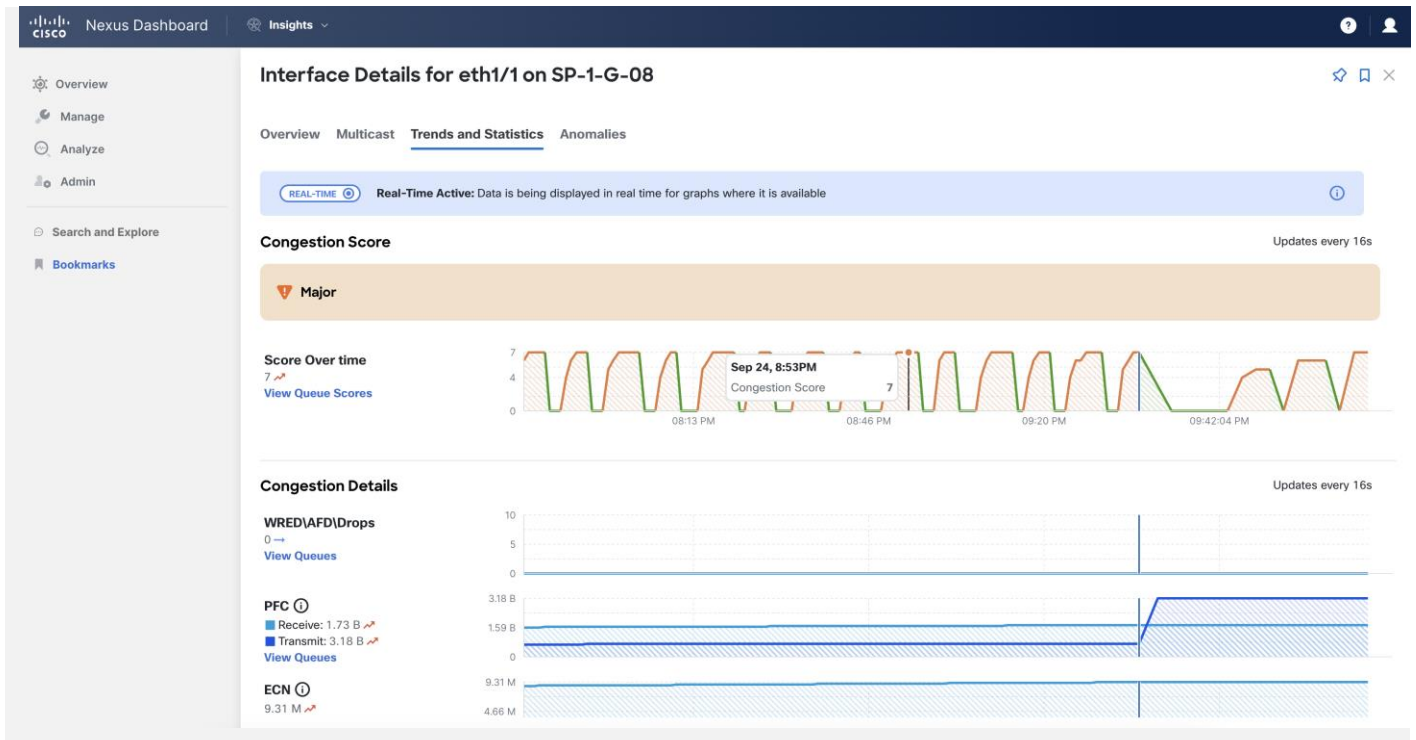
Figure 7. Nexus Dashboard identifies the severity of network congestion by calculating a congestion score
