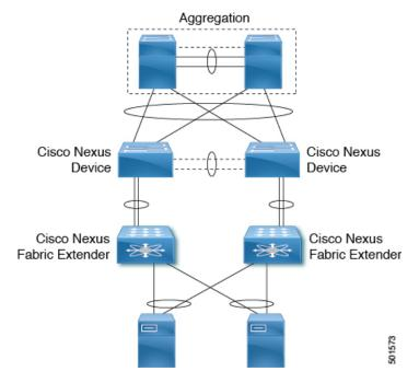
**Cisco Nexus Device Connected to Downstream Switches**
