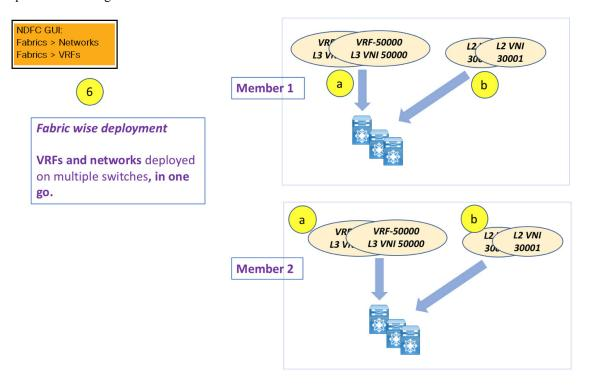
You can provision overlay networks through a single MSD deployment screen.
