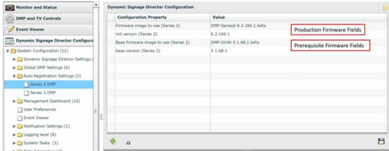
Figure 24 Firmware Image and Version Properties Required to Provision the SV-4K and DMP-2K
