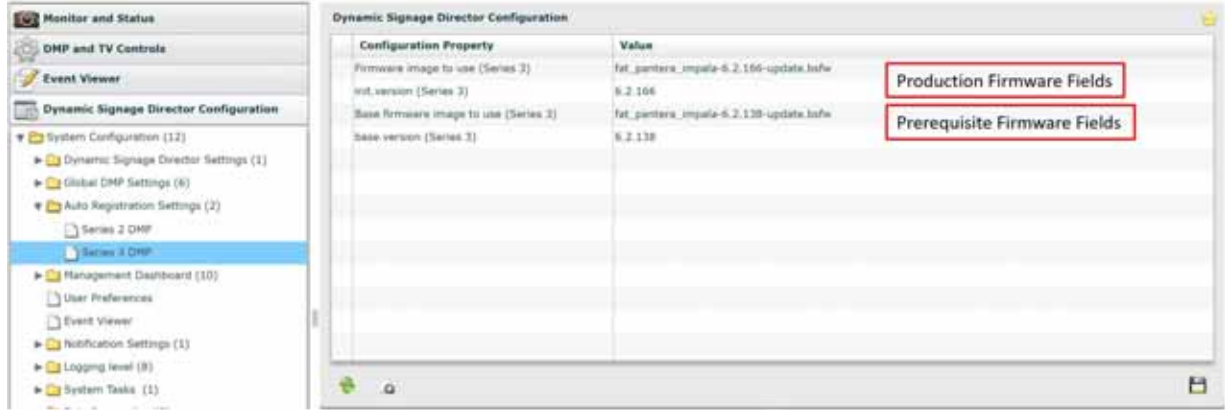
Figure 23 Firmware Image and Version Properties Required to Provision the CV-UHD and CV-HD
