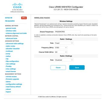
2. In the WIRELESS RADIO section, choose Radio 1 Role as Fluidmax Primary with FluidMAX Cluster ID. In this scenario, the frequency selection for the Primary is enabled and Secondary is disabled. In the ADVANCED RADIO SETTINGS window, go to Max TX Power section, and choose power level as 1 from the Select TX Max Power drop-down list and URWB transmission power control (TPC) automatically selects the optimum transmission power.
