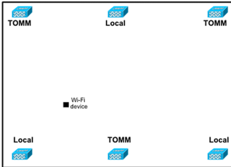
Figure 10: Tracking Optimized Monitor Mode AP deployment
